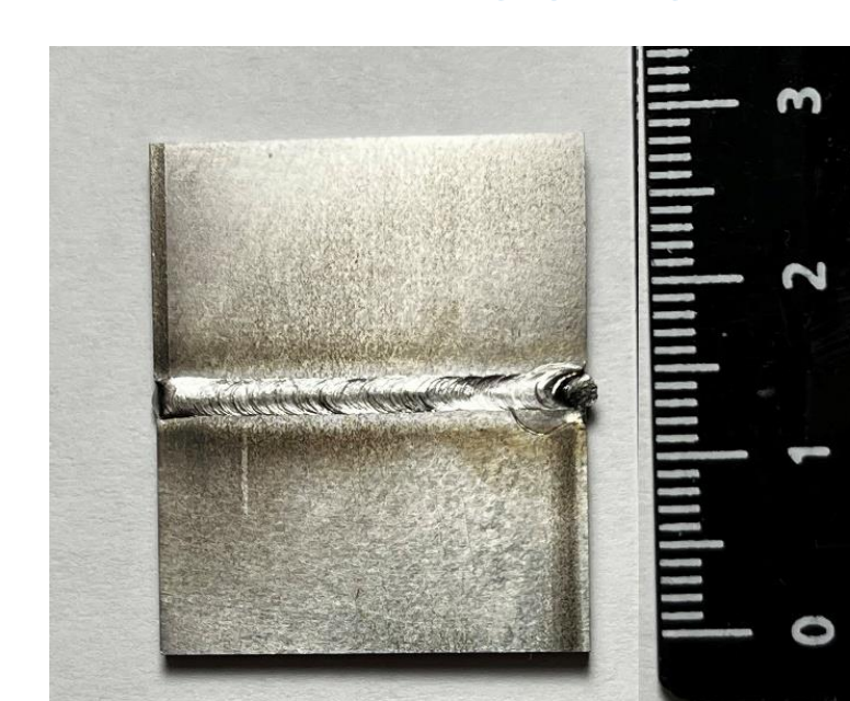
Figure - 23. Appearance of the welded joint obtained by EBW and tensile graph of welded joints
