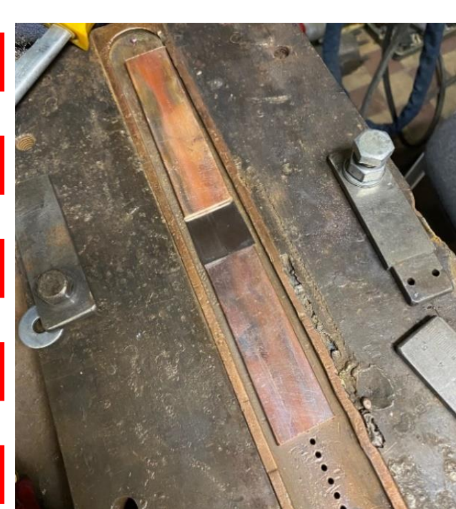
Figure - 13. TIG-welding equipment and GTAW modes of VTi-4 alloy plates, blowing gas and gas to burner = 15 l/min
