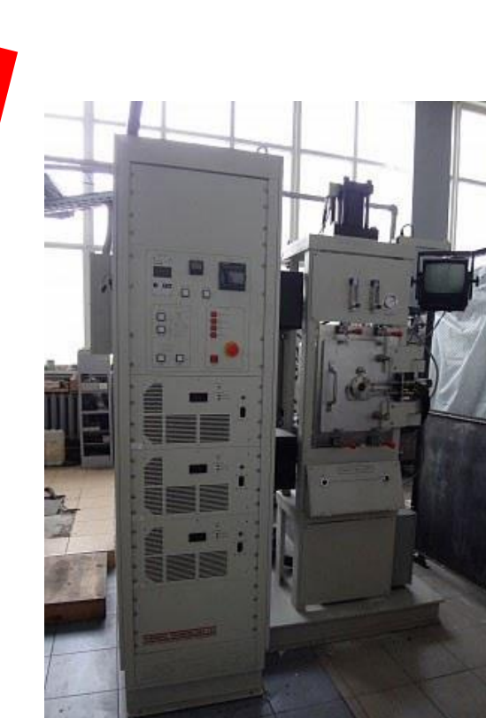
Figure - 17. Equipment SPS 10-3 for diffusion welding in vacuum (10 -4 Torr)
