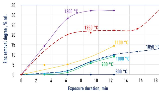
Dependence of zinc removal degree from EAF dust on the temperature and exposure duration when heated in the Tamman furnace in the argon current
