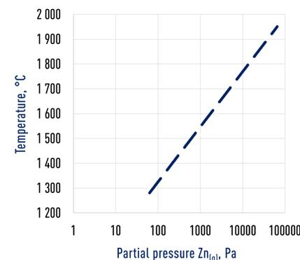
Dependence\* of the reaction temperature ZnO = Zn(g) + O<sub>2</sub>(g) on the partial pressure Zn(g)
