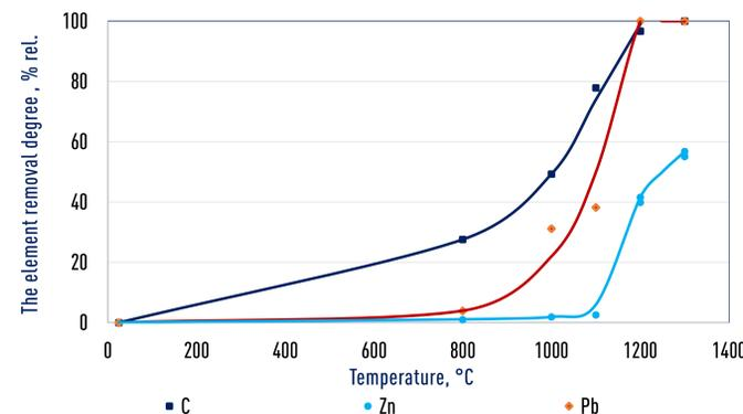
Dependence of the element extraction degree on the temperature during heating in the vacuum resistance furnace in the argon current
