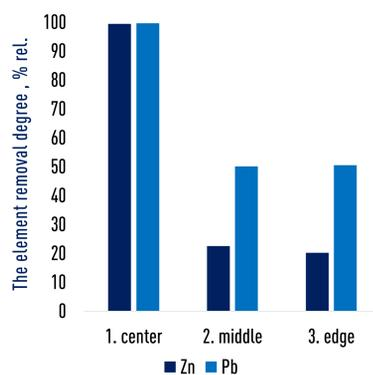
The dependence of Zn and Pb removal degrees from EAF dust during plasma treatment from the location
