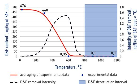
Change of dioxins and furans (D&F) content during EAF dust heating in the air atmosphere
