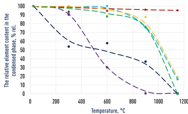
Pb, C, Na, Cl, K, Zn content change during heating of EAF dust in the air atmosphere
