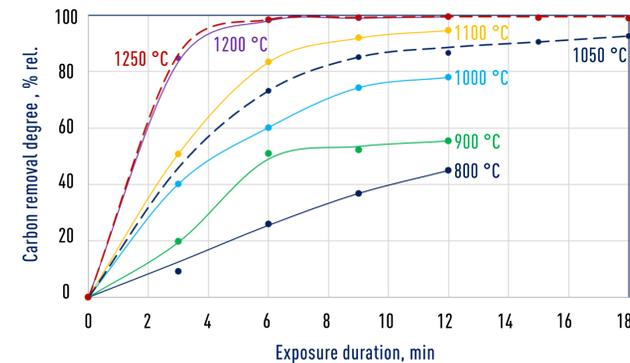
Dependence of carbon removal degree from EAF dust on the temperature and exposure duration when heated in the Tamman furnace in the argon current
