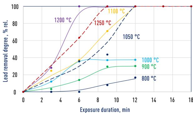
Dependence of lead removal degree from EAF dust on the temperature and exposure duration when heated in the Tamman furnace in the argon current
