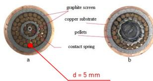
Scheme of samples placement on a substrate before (a) and after (b) plasma treatment
